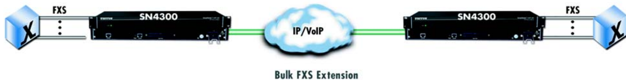
Figure 5. Bulk analog line extensions application
