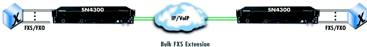
Figure 5. Bulk analog line extensions application
