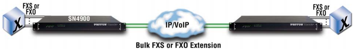
Figure 6. Bulk analog line extensions application
