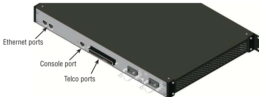
Figure 3. SmartNode 4900 rear panel ports
