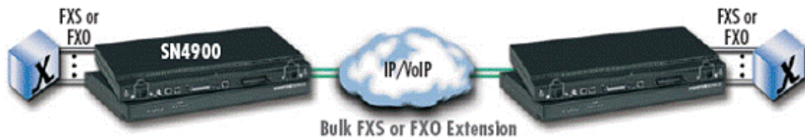
Figure 6. Bulk analog line extensions application
