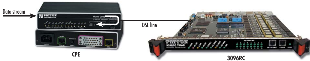
Figure 58. CPE local loopback
