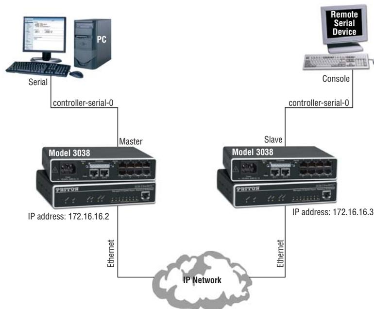
Figure 1. 3034/3038 networking diagram
