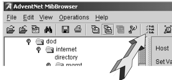
Figure 28. ManageEngine MibBrowser Settings Button on the Toolbar
