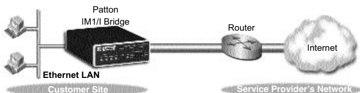
Figure 2. Cisco router with serial interface, configured as PPP Half Bridge.
