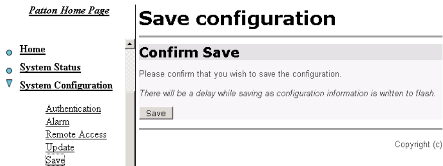
Figure 7. Save the configuration in non-volatile memory
