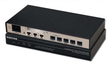
located with the server. For single-site enterprises, installing the gateway adjacent to the PSTN connection avoids the cost and hassle of pulling additional cable to the data center where the server resides. For multi-site enterprises, VoIP gateways eliminate the cost of buying and installing servers for every branch. A single server at headquarters can support each branch-office gateway through the IP network.
