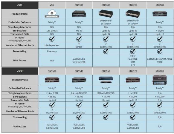
Remark: Limitation concerning the virtual SN (vSN) and SN5600 -> no transcoding and no SRTP available (models without DSPs). Support of SRTP planned in a future Firmware release.
