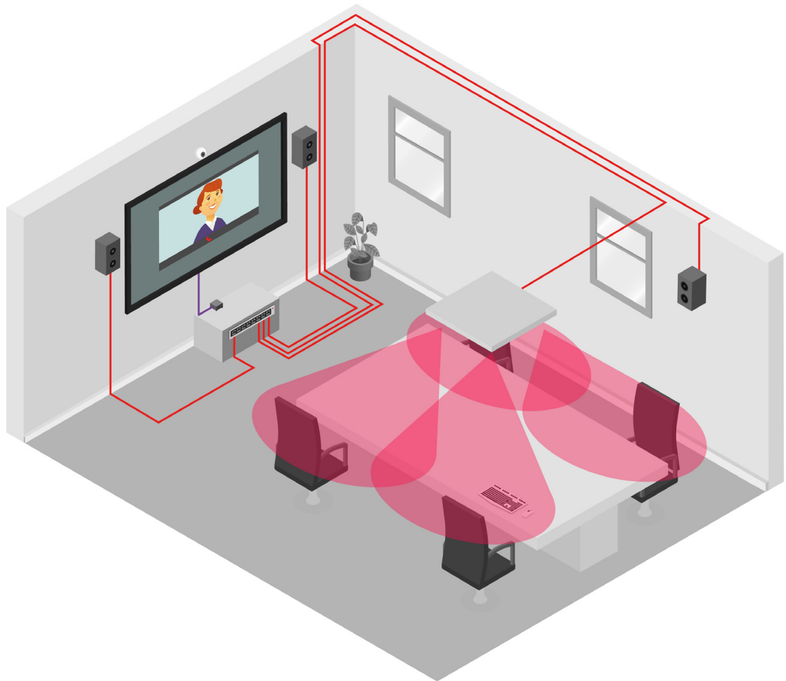
Figure 2: : Audio-over-IP solution with ceiling microphone and multiple loudspeakers for complete coverage
