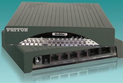
Patton's 1069 VDSL2 CPE offers the extraordinary bandwidth of 100-Mbps symmetrical over ordinary telephone grade copper wire for delivering next-generation Triple Play services.
