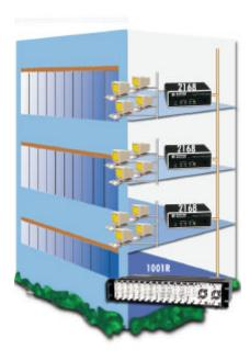
Used in pairs, the Patton Model 2168 establishes a high-speed (up to 16.67Mbps) communications link inter-connecting two geographically separated LANs or network enabled devices. Operation is simple: packets destined for the remote LAN are sent transparently, at full line rate, to the peered LAN. CopperLink Ethernet Extenders utilize ordinary voice-grade wire thus eliminating the cost and common barriers associated with installing new cable or expensive fiber.
