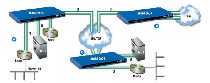
T1/E1 Aggregation. Medium-size enterprises can aggregate and groom time slots from up to three partially used local T1/E1 lines onto a single outgoing link. This capability enables routers, MUXs, and other network devices dispersed over the campus area to efficiently use a single T1/E1 line for network access.
