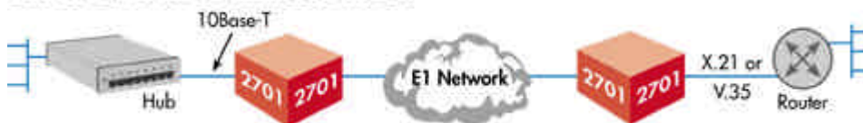
LAN-to-LAN Over E1 Without a Router
