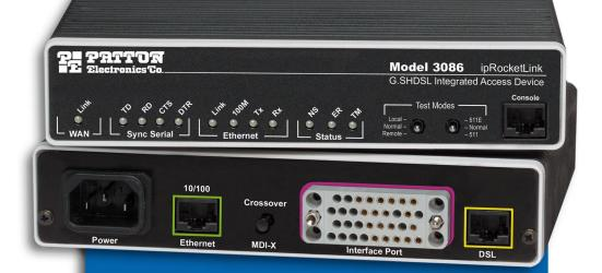
Based on the ETSI and ITU G.SHDSL G.991.2 standard, the Patton Model 3086 ipRocketLink IAD enables nx64 2.3/4.6 Mbps speeds over a single pair of wires while combining standards-based transmission with synchronous-serial, Ethernet, and high speed IP routing...all in one compact package.
