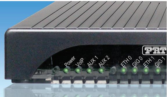
The SmartNode 5500 Series of Enterprise Session Border Controllers supports up to 200 SIP-to-SIP calls (up to 16 of which can be transcoded\* SIP to SIP calls). Service demarcation is key for high quality and reliable services, even in All-IP networks. State-of-the-art security and quality guaranteed.
