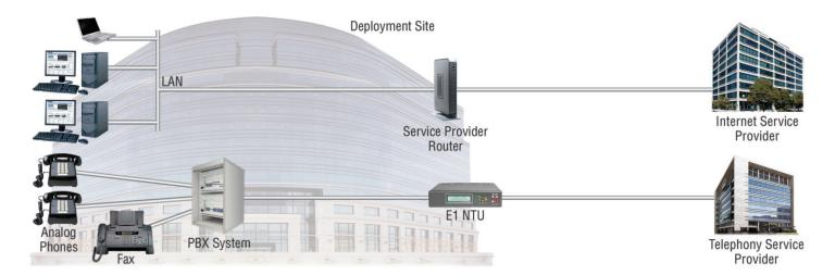
With introduction of NBN, the service provider router talks over the NBN layer-II IP network.
