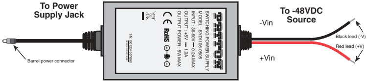
Figure 5. Connecting DC Power to the 2701 DC Power Supply.
