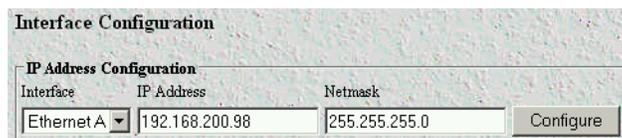
Figure 17. Interface configuration window
