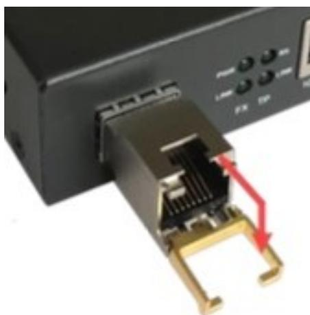
2. Remove the module from the slot of the main unit (Figure 7).
