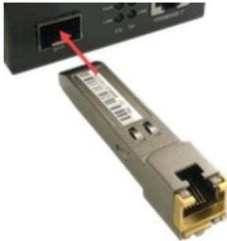
2. Apply some pressure on the module. When it is properly inserted (Figure 5) you'll hear a distinctive sound.
