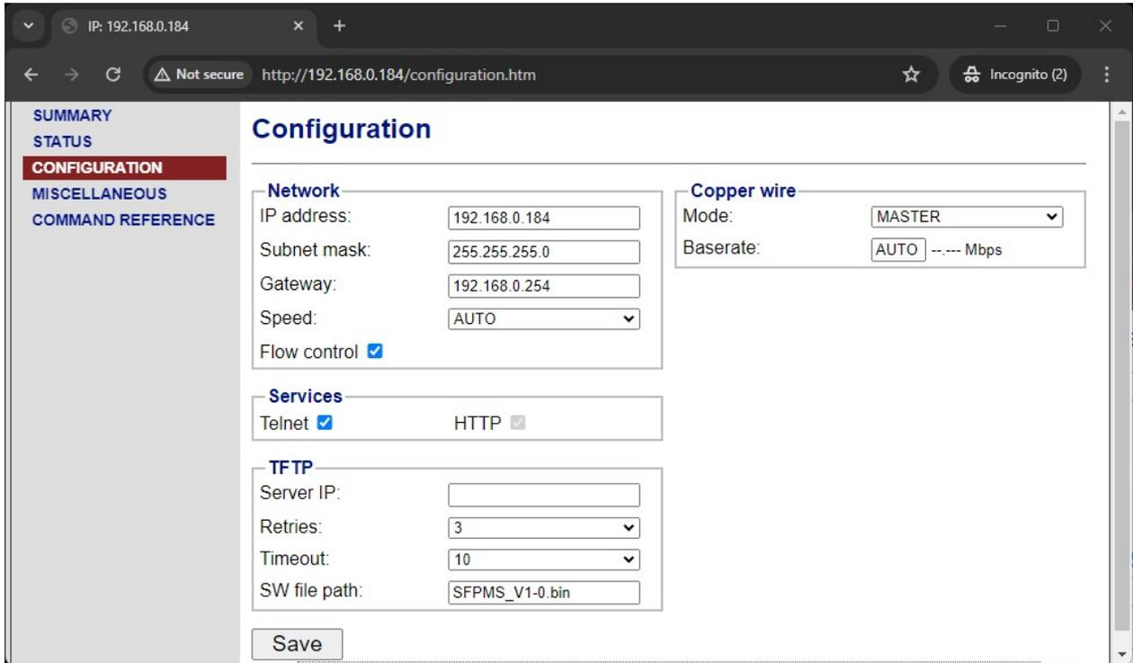
FIGURE 3.20 EXAMPLE CONFIGURATION OF MASTER MODEM IN AUTO RATE MODE (WEB)
