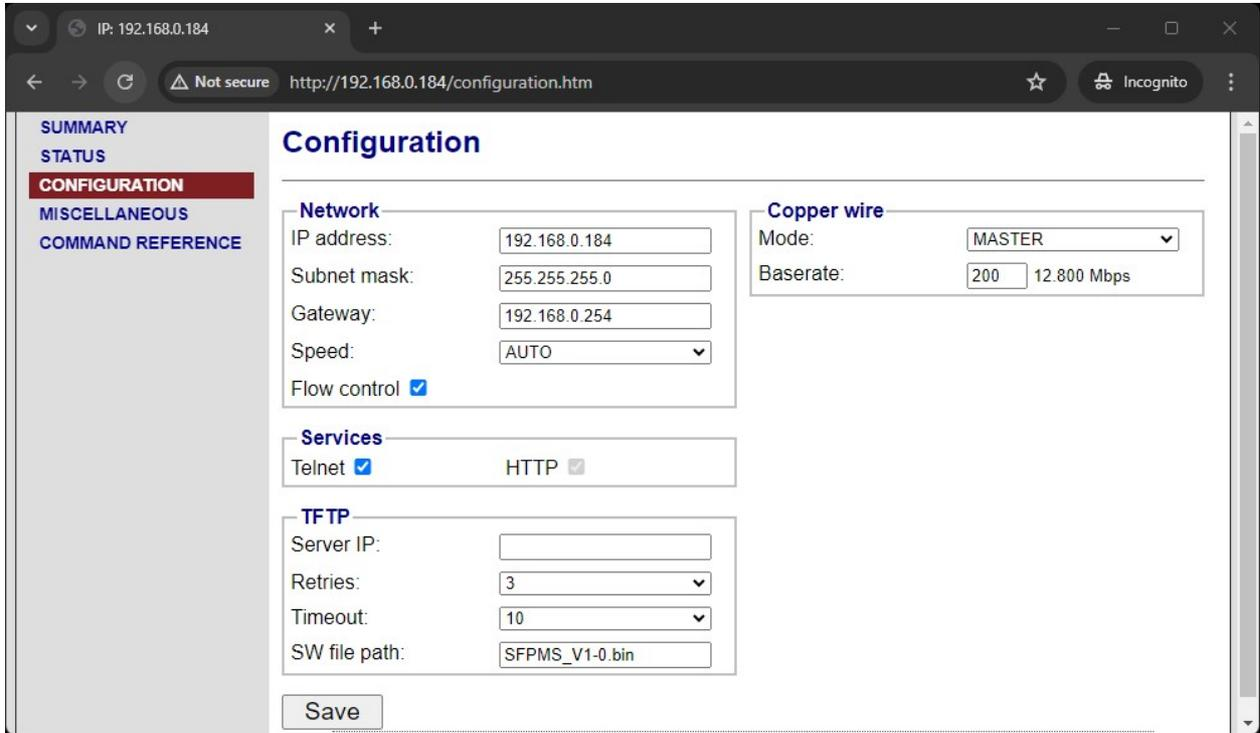
FIGURE 3.12 EXAMPLE CONFIGURATION OF MASTER MODEM IN FIXED RATE MODE (WEB)
