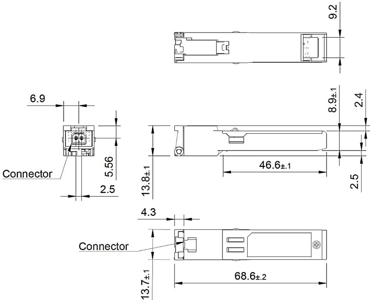
FIGURE 4.2 CL-SFP/XC DIMENSIONS
