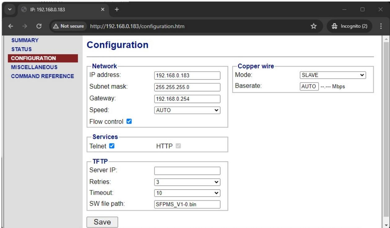
FIGURE 3.21 EXAMPLE CONFIGURATION OF SLAVE MODEM IN AUTO RATE MODE (WEB)
