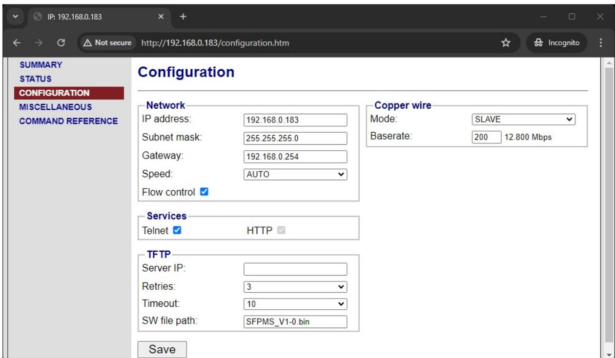
FIGURE 3.13 EXAMPLE CONFIGURATION OF SLAVE MODEM IN FIXED RATE MODE (WEB)
