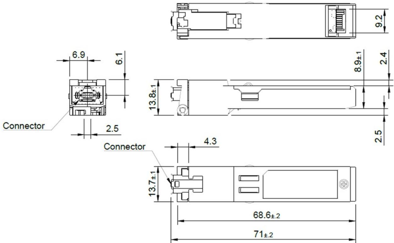
FIGURE 4.5 CL-SFP/SPE DIMENSIONS
