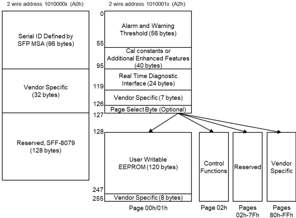
FIGURE 5.1 DIGITAL DIAGNOSTIC MEMORY MAP SPECIFIC DATA FIELD DESCRIPTIONS
