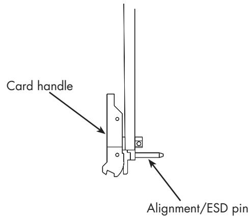
Figure 7. Alignment/ESD pin on card handle
