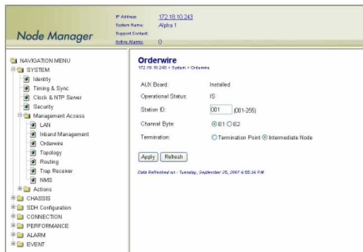
Figure 22. Configuring the Engineering Orderwire (EOW) Function
